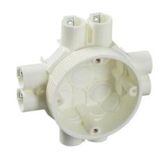
The AU8 junction box is 53 mm high and has eight inlets for Ø 20 conduits. The box also has knock-outs for 4 side inlets and 4 bottom inlets. In wall installation the box can be attached with a AS13.12 support. Made of halogen free material (IEC/61249-2-21) and fulfills the requirements of the glow wire test according to the standard IEC/EN60670: 2005 (850 °C). Max amount of conductors 30.
