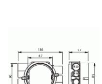
Manufactured from halogen free material (IEC/61249-2-21), the box complies with the IEC/EN60670:2005 glow wire test (850 °C).
